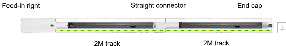
4 metre straight run made with two lengths of 2 metre track and a straight connector. Power is provided through the feed-in which is an earth right, therefore the earth runs along the right side of the track. Termination of the track is achieved by the end cap, which has no polarity.
