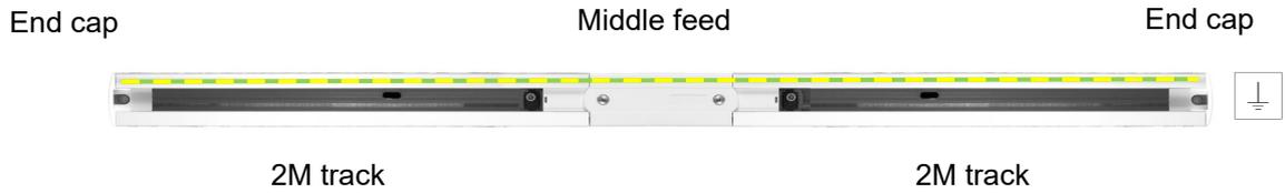
4 metre straight run made with two lengths of 2 metre track and a middle feed. Power is provided by the middle feed, which can be turned around to allow the earth to be either side. Termination of the track is achieved by end caps on both ends.
